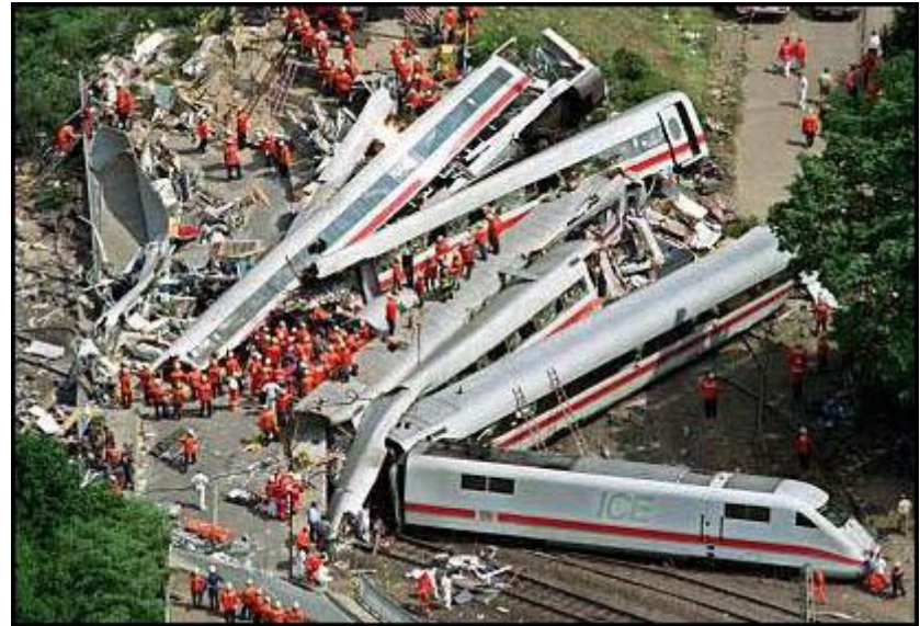
June 3, 1998 : failure of the tread of a wheel of an ICE 1 from Munich to Hamburg
