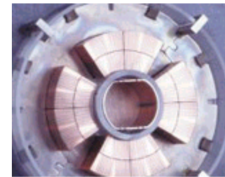
Quadrupoles are used for beam focusing
